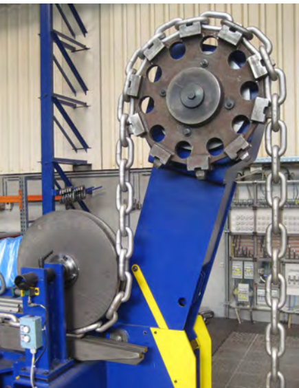
Above: Chain links are tested for dimension in the most modern sensor-controlled machines and, if need be, their tolerance range is extended. Their perfect sprocket fit is checked at this point before the chain reaches the hardening stage.
