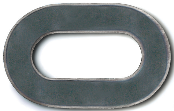
Cross section through case hardened chain link
