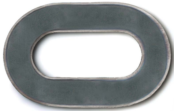
Cross section through case hardened chain link
