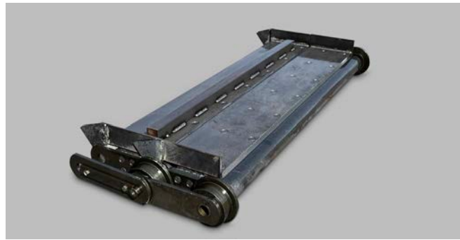
Figure 4. Chain segment of modified apron conveyor chain.
