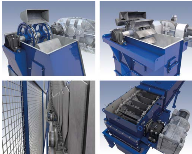
Figure 5. Examples of standardised conveyor chains – wear-resistant round link chains (upper left), central chains for high-performance bucket elevators (upper right), pan conveyor chains (lower left), and forged link chains (lower right).
