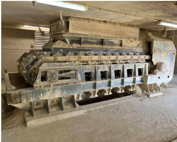
Figure 1. Heavy duty apron conveyor for limestone hopper discharge.
