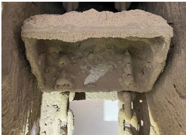
Figure 3. Wet sand caking on chain and buckets.
